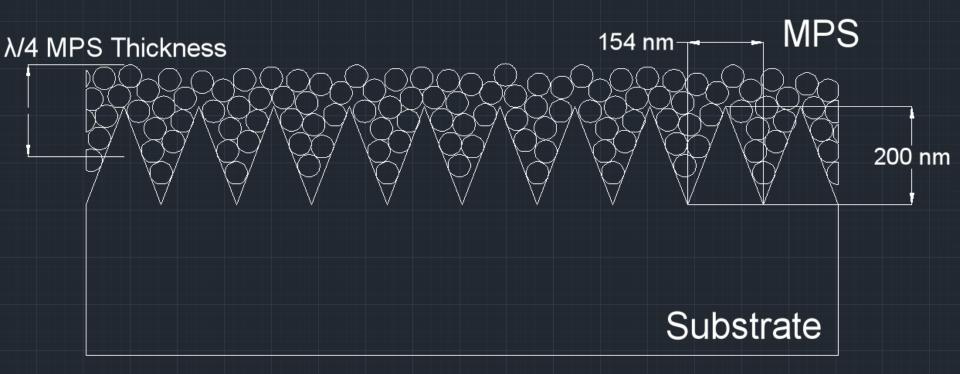
MPS passivation film  $\lambda$  /(4 n<sub>MPS</sub>) film thickness NS - AR coating and MPS bonding site
